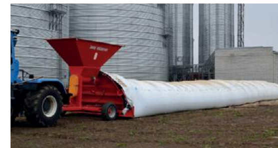
Length of bag 60 m with capacity 200 t. of grain
