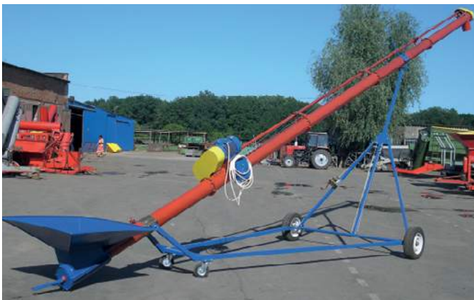
Stationary auger SSH-250/12,5 with adoptive bunker
