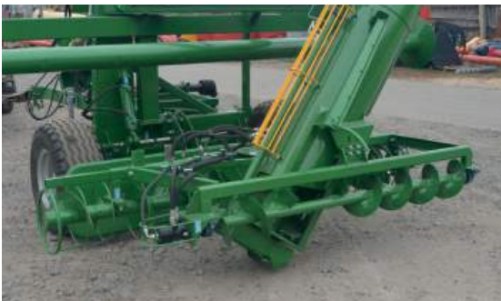
Additional horizontal auger for corn
