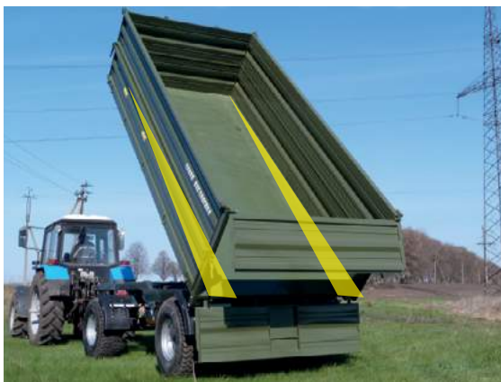
Conical body prevents jam of green mass and fertilizers
