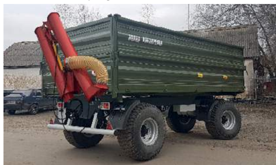
Back wall adopted for reloading auger
