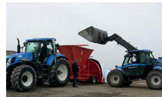
Packing grain in to the bag with ZPM-180P
